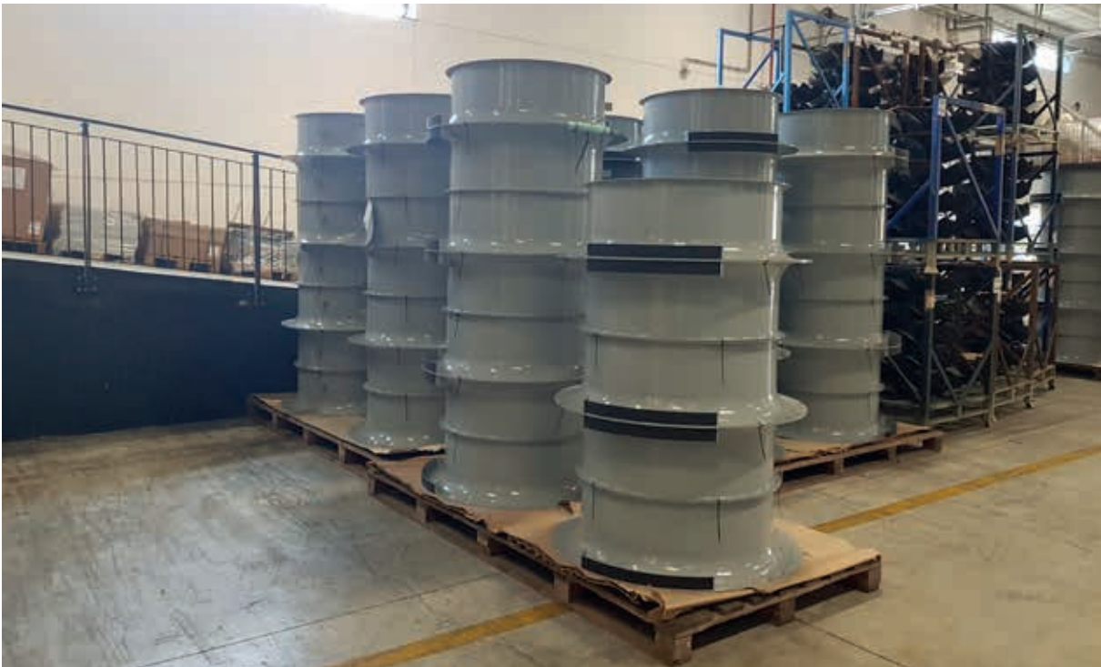
Turbine pipes and intake ports after delivery
