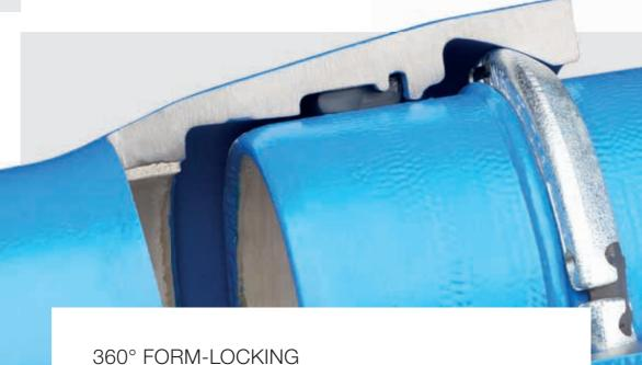
Full form-locking joints to 360°. Ductile iron cast pipe from the ALPINAL system have TIS-K restrained socket joints. The retaining ring does not work on just one or two sides of the pipe but around the full 360°. Consequently, the stress is distributed evenly along the joint.
