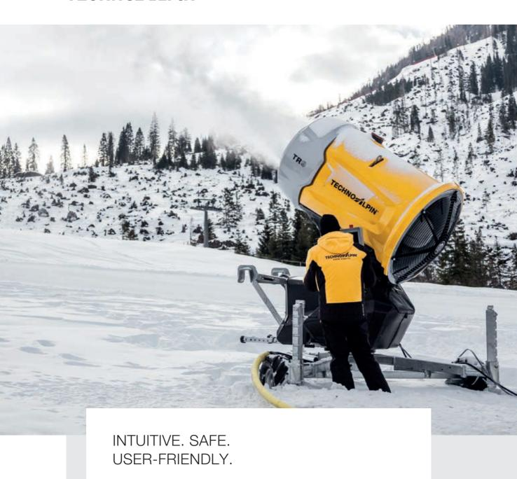
The TR9 features automatic height adjustment and swinging function to facilitate the work of the snowmaking team. Thanks to the optimized design, all components are easily accessible and the device is easy to handle. The TR9 is also impressive because of its touch display – the biggest on the market.
